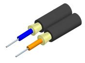
Fiber indoor cable, 1.6 mm diameter, Plenum rated, Zipcord 2-fiber, Singlemode G.657.A2/B2, Feet jacket marking, Black jacket color
