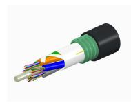
Fiber OSP cable, LazrSPEED® Single Jacket/Single Armor, Gel-Free, Stranded Loose Tube, Multimode OM3, Feet jacket marking, Black jacket color
