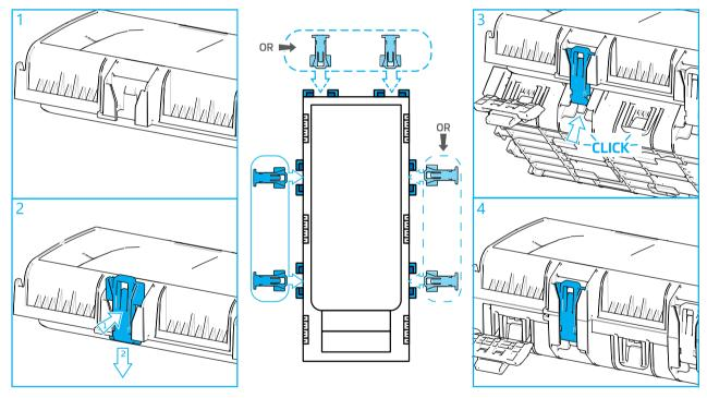
The hinges can be installed on the left, right or at the top of the cover.
