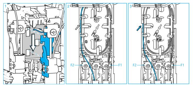
1 Prepare the cable as explained in the section 'Feeder cable preparation'. Verify in section 'Port reducers' if the port reducers should be removed. Insert the branch cable in the middle position on the rear side.
