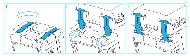
**Note:** If the hinges are installed in the top position, the cover **cannot be secured in open position**. To access the inside of the closure, the cover should be detached.
