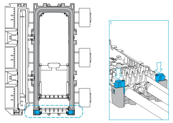
1 Position the organizer in the closure with the front side (drop side) facing on top. Push firmly on the snap features to lock the organizer in the closure. When a click sound is noticed, the organizer is properly locked.
