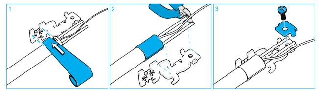
1 If the diameter is smaller than 9 mm (0.35 Inches) or if the jacket is a thin jacket, add 5 wraps of self amalgamating silicon tape. Stretch the tape between 50% and 300% while wrapping the tape around the cable. Make sure the tape is wrapped where the hose clamp will be positioned.
