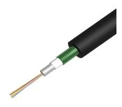
Fiber OSP cable, PE, Gel-filled Central Tube, CST, 12 fiber, Multimode OM5, Meters jacket marking, Black jacket color
