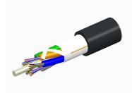
Fiber indoor/outdoor cable, TeraSPEED®, Single Jacket All-Dielectric, Low Smoke Zero Halogen (LSZH), 6 fiber, Singlemode G.652.D and G. 657.Al, Gel-Free, Stranded Loose Tube, Black jacket color, Meters cable marking, Eca flame rating
