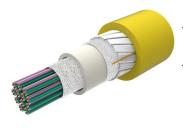
Fiber indoor cable, All-Dielectric, LSZH/Riser-Rated, Gel-Free, Central Tube 200µm Rollable Ribbon, 432 fiber, Singlemode G.657.A2/B2, Feet jacket marking, Yellow jacket color, Cca flame rating
