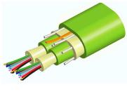
Fiber indoor cable, LazrSPEED® Low Smoke Zero Halogen Riser MPO Trunk, 16 fiber with 8 fiber 2.0mm subunits, Gel-free, Multimode OM5, Meters jacket marking, Lime green jacket color, B2ca flame rating
