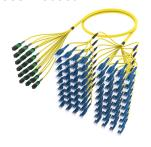
Singlemode MPO8 APC non-pinned to LC/UPC Uniboot Ruggedized fanout Cable, 144-Fiber, LSZH, 8 fiber PmP 2.0 mm /B2ca
