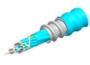
Fiber indoor cable, Riser/LSZH rated, MPO Trunk, interlocking aluminum armored, OM4 multi-mode, 128 fiber, Feet jacket marking, Aqua jacket color, B2ca flame rating
