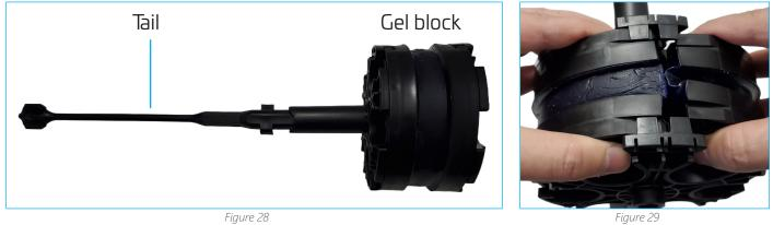
10.2 Position the gel block against the spacer on the star bracket. Position the cables and snap the gel block closed. **Warning**: Do not use a braided or stranded ground wire when installing ground wire through a port on the FOSC450 closures. To prevent a leak path, only a bonded solid ground wire with sealing kit is to be used. Refer to the external ground wire installation manual for more details.
