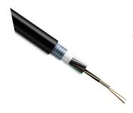
Fiber Optic Outdoor 24 Fiber Multi-tube Cable with Corrugated Steel Armoring, OM3, with HDPE Jacket
