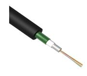
Outside Plant Fiber Optic Cable, HDPE, 8-fiber, Multimode, OM3, loose tube, gel-filled, 2000 m
