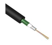
Outside Plant Fiber Optic Cable, HDPE, 24-fiber, OS2, loose tube, gel-filled. Provides Rodent Resistance.
