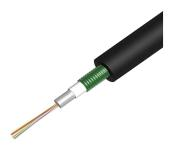
Fiber indoor/outdoor drop cable, LSZH, Gel-filled Central Tube, CST, 4 fiber, Multimode OM4, Meters jacket marking, Black jacket color
