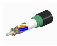
Fiber OSP cable, LightScope ZWP® Single Jacket/Single Armor, 288 fiber, Gel-Free, Stranded Loose Tube, Singlemode G.652.D and G.657.Al, Meters jacket marking, Black jacket color
