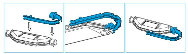
1 Install the fiber cable guide as shown in the pictures above until it snaps onto the SRC10.
