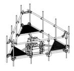
3-Sector Monopole Co-location Platform Kit, 10 in to 30 in OD, 14 ft 6 in face, includes twelve 96 in pipes
