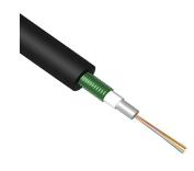
Fiber Optic Outside Plant Cable, 6-core, CST (Corrugated Steel Tape) Armored, Loose-tube, Gel-filled, 50/125 µm, OM4, Multimode, Black cable jacket
