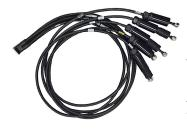
HELIAX® M-LOC Multiport cluster 5 ports SureFlex® cable assembly with Integrated Birdproofing Shell with interface type M-LOC latching male to 4.3-10 male with HELIAX® SureGuard weatherproofing on 4.3-10 end, size 1/4", length 3 meters,
