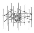
G23RHDX Monopole Sector Frame with spine extension for RRU Mounting,  $10.5 \, \text{ft} \times 2.88 \, \text{in OD}$  face pipes, includes nine  $2.88 \, \text{OD} \times 120 \, \text{in}$  antenna pipes
