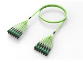
Ultra Low Loss (ULL) OM5 MPO16 (Pinned) to MPO16 (Pinned), Fiber Trunk Cable Assembly, 192-Fiber, Dual Rated (OFNR/LSZH)
