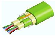
Fiber indoor cable, LazrSPEED® Low Smoke Zero Halogen Riser MPO Trunk, 16 fiber with 8 fiber 2.0mm subunits, Gel-free, Multimode OM5, Meters jacket marking, Lime green jacket color, B2ca flame rating
