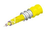
Fiber indoor cable, TeraSPEED® Plenum MPO Trunk, interlocking aluminum armored with plenum jacket, Singlemode G.652.D and G.657. Al, 144 fiber multi-unit with 12 fiber subunits, Yellow jacket color, Feet cable marking
