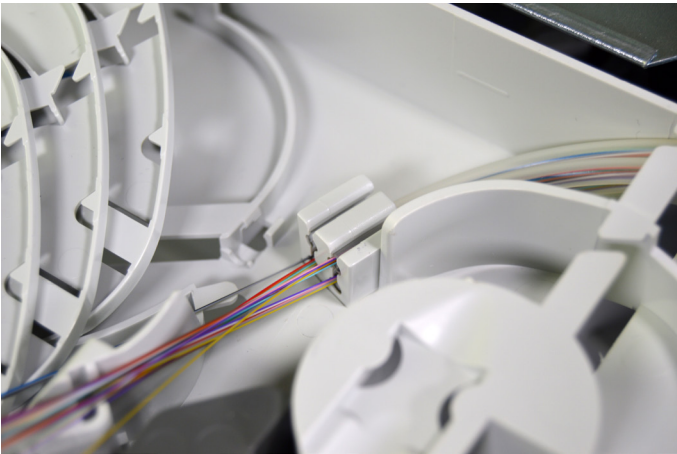
6.1.9. Push and click the tube holder into the tray. Route the transportation tubes into the FACT element.
