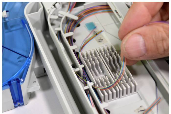
7.2.6. Guide the fibers into the splice island.
