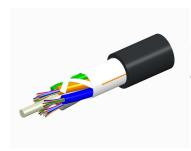
Fiber OSP cable, LightScope ZWP® Single Jacket All-Dielectric, Gel-Free, Outdoor Stranded Loose Tube, 288 fiber, Singlemode G.652.D and G.657. Al, Feet jacket marking, Black jacket color
