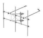
G23HDX High Capacity Sector Frame,12.5 ft x 2.88 in OD face pipes, includes three 2.88 OD x 120 in antenna pipes
