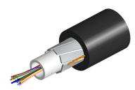
Outdoor Fiber Optic Cable, 6-fiber, multimode, OM4, PE, loose tube, gel-filled, cut length
