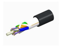
Fiber indoor/outdoor cable, LazrSPEED®, Single Jacket All-Dielectric, Low Smoke Zero Halogen (LSZH), 36 fiber, Multimode OM4, Gel-Free, Stranded Loose Tube, Black jacket color, Meters cable marking, Eca flame rating
