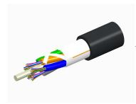
Fiber indoor/outdoor cable, LazrSPEED®, Single Jacket All-Dielectric, Low Smoke Zero Halogen (LSZH), Gel-Free, Stranded Loose Tube, 36 fiber, Multimode OM3, Black jacket color, Feet cable marking, Eca flame rating
