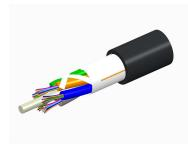
Fiber indoor/outdoor cable, LazrSPEED®, Single Jacket All-Dielectric, Low Smoke Zero Halogen (LSZH), 96 fiber, Gel-Free, Stranded Loose Tube, Multimode OM3, Black jacket color, Meters cable marking, Eca flame rating
