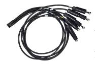
HELIAX® M-LOC Multiport cluster 5 ports SureFlex® cable assembly with Integrated Birdproofing Shell with interface type M-LOC latching male to 4.3-10 male with HELIAX® SureGuard weatherproofing on 4.3-10 end, size 1/4", length 2 meters,
