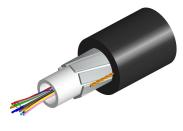
Fiber OSP cable, Single Jacket All-Dielectric, 8 fiber Gel-Filled, Outdoor Central Tube, Singlemode G.657.A1, Meters jacket marking, Black jacket color
