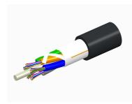
Fiber indoor/outdoor cable, TeraSPEED®, Single Jacket All-Dielectric, Low Smoke Zero Halogen (LSZH), 12 fiber, Singlemode G.652.D and G. 657.A1, Gel-Free, Stranded Loose Tube, Black jacket color, Meters cable marking, Eca flame rating
