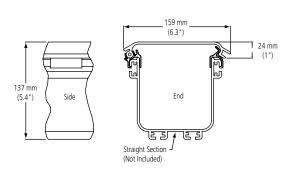
Hinged Cover for 4" Horizontal Straight Section (FGS-MSNC-A)
