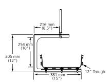
Top Support Threaded Rod C-Bracket Kit (FGS-HNTS-F-XX shown attached to 4x12 straight section)
