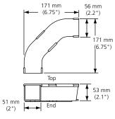
90° Extended Horizontal Elbow (FGS-MH9A-C-45/2)
