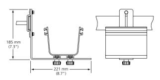
Ladder Rack Cantilever Support Bracket Kit (FGS-HDLB-4)
