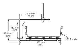
Top Support Low Profile Threaded Rod C-Bracket Kit (FGS-HNTS-F-XX-LP shown attached to 4x12 straight section)
