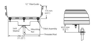
Center Support Threaded Rod Bracket Kit (FGS-HTUB-F-XX shown attached to 4x12 straight section)
