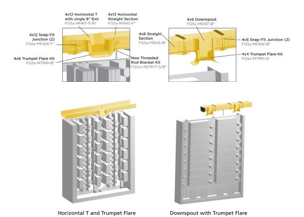
When attaching a straight section or fitting to the exit of a 4x4 or 4x6 downspout, the FGS-MJWR-A junction must be used. This junction is only required to connect the vertical part, the FGS-MFAW-x junction can be used to connect the horizontal parts.
