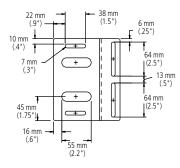
OMX Frame Center Support Bracket Kit (FGS-HOMX-16MM)
