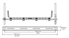
New 5/8" Threaded Rod Trapeze Bracket Kit (FGS-HNTP-H-5/8)
