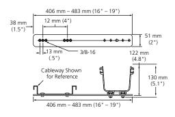
Digital Cableway Bracket Kit (FGS-HCBL shown alone and attached to 4" FiberGuide®)
