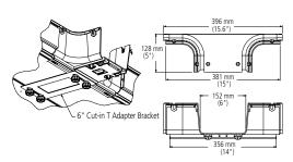
6" Cut-in T designed exclusively for the 4x24 System (FGS-MHIS-B/H)
