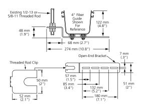
Modified Existing Threaded Rod Bracket Kit (FGS-HETR-XX-A shown alone and attached to threaded rod)
