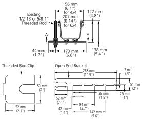
Existing Threaded Rod Bracket Kit (FGS-HETR-XX shown alone and attached to threaded rod)
