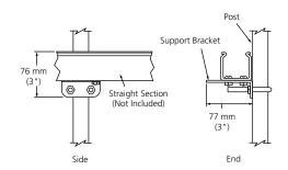
Under Floor Support Kit (FGS-HUFB-C shown attached to .62"x 2" round pipe)
