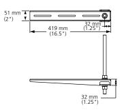
New Threaded Rod Bracket Kit (FGS-HNTR-F-XX shown alone and attached to threaded rod)
