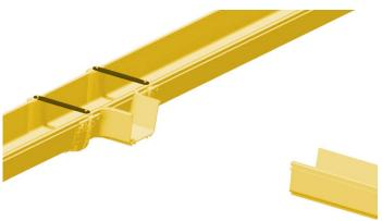
Raceway system with gap between opposing runs
