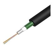
Fiber OSP cable, PE, Gel-filled Central Tube, CST, 8 fiber, Multimode OM3, Meters jacket marking, Black jacket color
