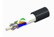
Fiber indoor/outdoor cable, TeraSPEED®, Single Jacket All-Dielectric, Low Smoke Zero Halogen (LSZH), Singlemode G.652.D and G.657.A1, 12 fiber, Gel-Free, Stranded Loose Tube, Feet jacket marking, Black jacket color, Eca flame rating
