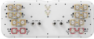
16-port sector/multibeam antenna 4x 694–960 MHz , 4x 1695-2690 MHz 65° HPBW and 8x 1710–2690 MHz 2x 2-Beam 33°HPBW, 8x RET. Band cascaded SRET
