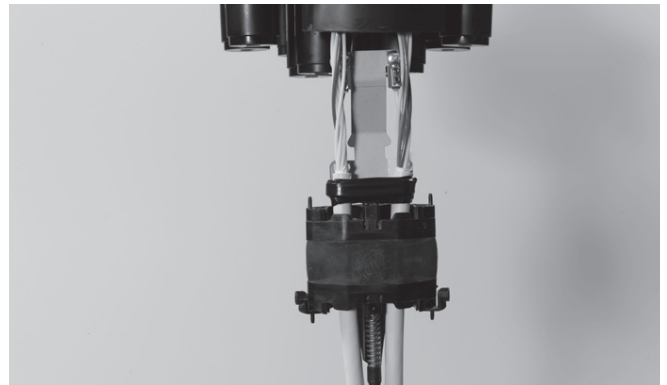
3.2.5 Insert the assembly as shown, metal bracket at the back of the cables!
