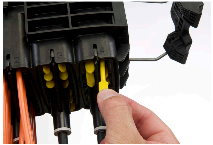
6.8 In case a cable needs to be added release the trigger and remove the dummy rod. To add a cable/ tube, release the trigger, remove the blind plug and prepare new cable as described above.
