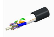
Fiber indoor/outdoor cable, TeraSPEED®, Single Jacket All-Dielectric, Low Smoke Zero Halogen (LSZH), Singlemode G.652.D and G.657.A1, 72 fiber, Gel-Free, Stranded Loose Tube, Meters jacket marking, Black jacket color, Eca flame rating
