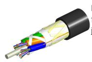
Fiber OSP cable, LightScope ZWP® All-Dielectric Self-Supporting, 60 fibers, 2.5mm Gel-filled Tubes, Singlemode G.652.D and G.657.Al, Meters jacket marking, Black jacket color
