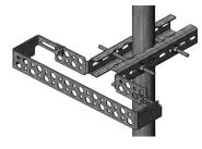
PIM-Guard® Antenna and RRU Cable Support Bracket with 23 ports for stackable hangers (up to 3 per port). Install with torque wrench set at 10 to 15 ft-lb to meet carrier PIM requirements. For patents, see www.cs-pat.com
