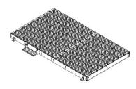
Equipment Platform, 8 ft x 14 ft, base with Pier Connections
