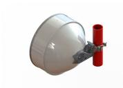
0.6 m | 2 ft Sentinel® High Performance Antenna, dual-polarized, 12.7 –13.25 GHz, PBR flange, white antenna, grey radome
