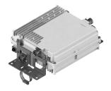
Tri Band Tower Mounted Amplifier, 1800/2100/2300 MHz, 12 dB, 2 BTS & 2 ANT ports, AISG with 1 RET connector (3 devices with 2 sub-units each)
