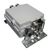
Dual Band Tower Mounted Amplifier, 2100//2600, 12 dB, 2 BTS & 2 ANT ports, AISG with 1 RET conector (1 device with 2 sub-units each)
