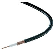
FSJ2-50, HELIAX® Superflexible Foam Coaxial Cable, corrugated copper, 3/8 in, black non-halogenated, fire retardant polyolefin jacket B2ca s1a d0 a1 Compliant
