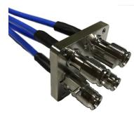
HELIAX® M-LOC Multiport cluster 5 ports SureFlex® cable assembly with interface type M-LOC female to open end, size 0.141", length 3.5 meters
