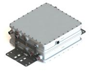
Tri Band Tower Mounted Amplifier, 1800/2100/2600 MHz, 12 dB, 2 BTS & 4 ANT ports, AISG with 1 RET connector (1 devices with 2 sub-units each), with 4.3-10 connectors, 698-960 MHz Bypass
