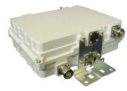
Dual Band Tower Mounted Amplifier, 1800//2600 MHz, 12 dB, 2 BTS & 2 ANT ports, AISG with 1 RET connector (2 devices with 2 sub-units) with improved Out of Band Tx rejection
